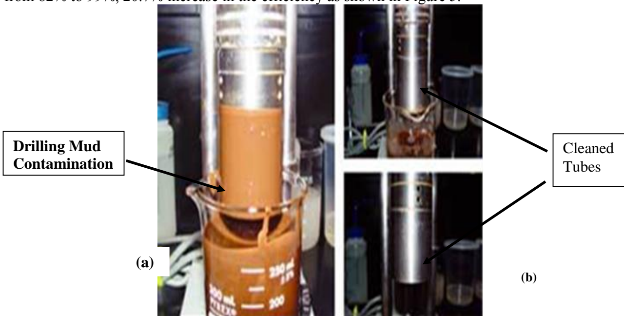
Figure 4 Cleaning Efficiency Test using Viscometer (a) Drilling Mud Contaminated Cylinder and (b) After Cleaning with the Spacer Fluid
