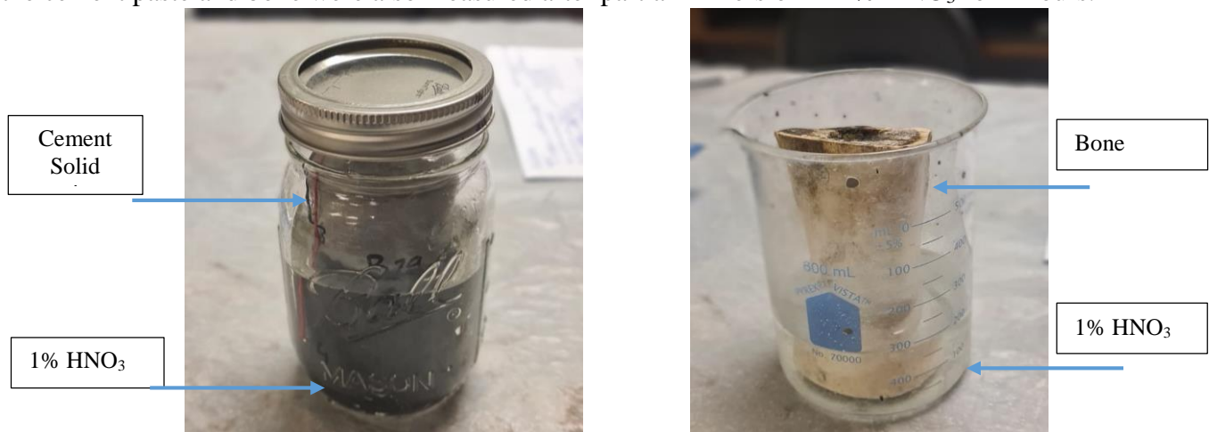
Figure 1: (a) Cement paste sample and (b) Bone sample, partially immersed in 1% Nitric Acid.
