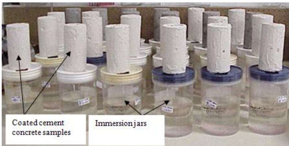
Figure 1. Specimens being dried for measuring the weight change during the drying cycle
