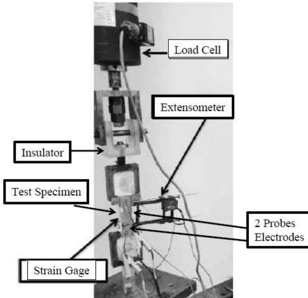
Figure 1. Direct Tensile Test Configuration.
