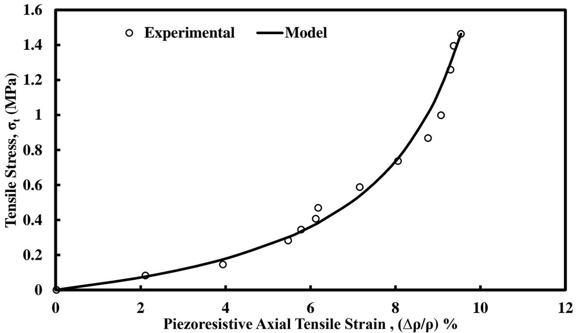
Figure 3. Direct tensile stress-piezoresistive axial strain response of cement after 28 days of curing
