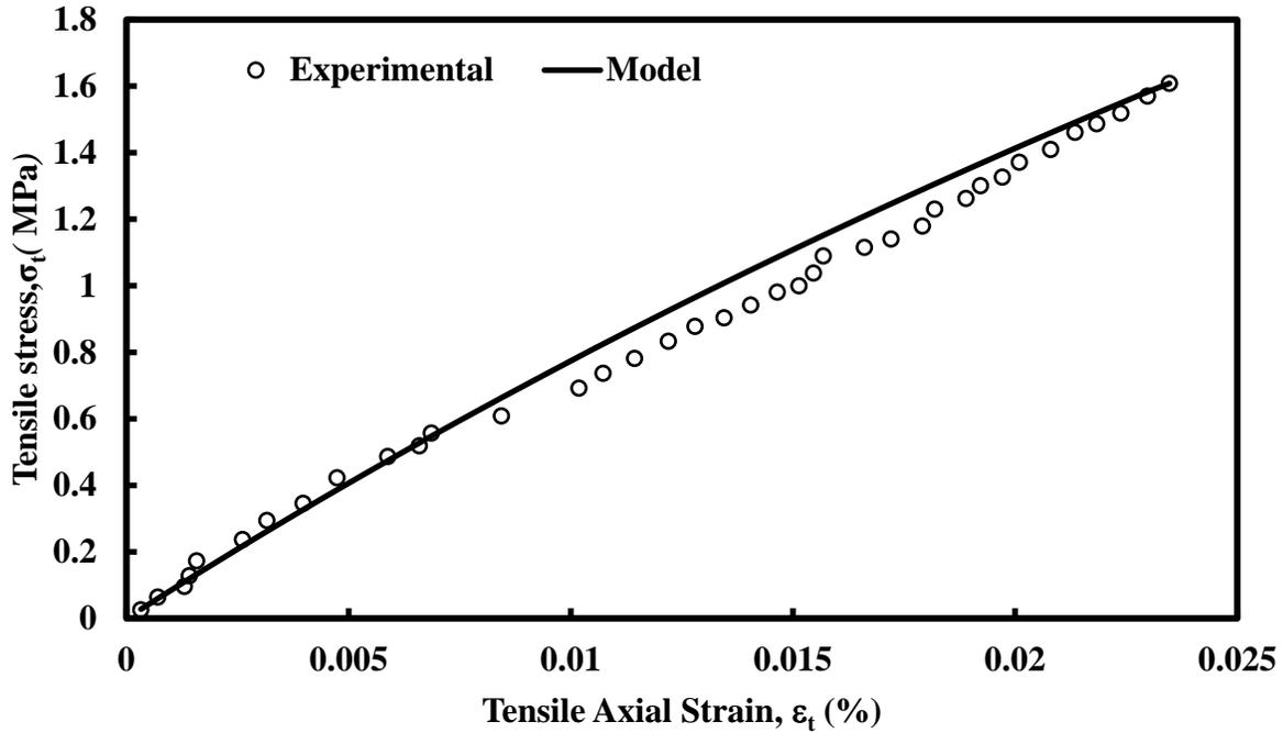
Figure 2. Direct tensile stress-strain response of cement after 28 days of curing
