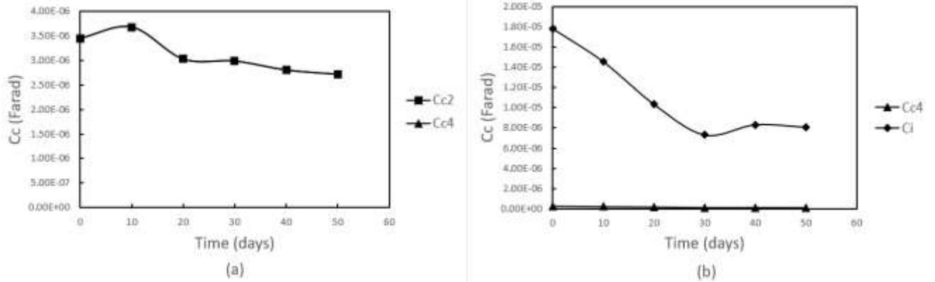
**Figure 12 Variation of contact capacitance of (a) C2-C4 probe configuration and (b) M1-C4 probe configuration over time**
