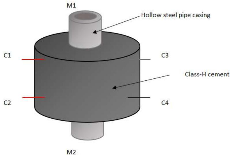
**Figure 7 Cement-steel casing with wire-probe configuration (C1, C2, C3 & C4 are the cement contact points and M1 & M2 are the steel casing contact points)**
