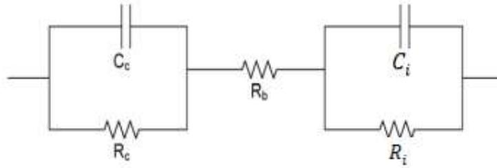
**Figure 8 Vipulanandan corrosion model for two probe measurements**
