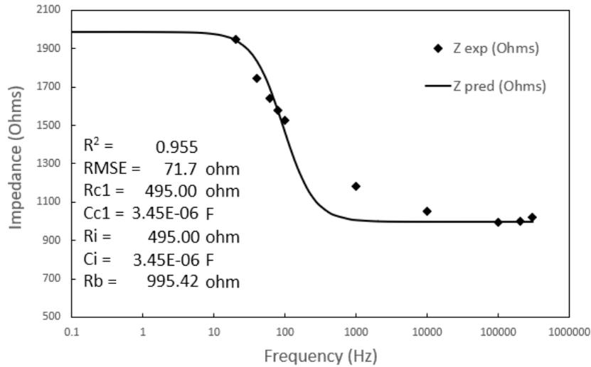
**Figure 9 Impedance versus frequency plot of C2-C4 probe configuration on day 1 of corrosion test**
