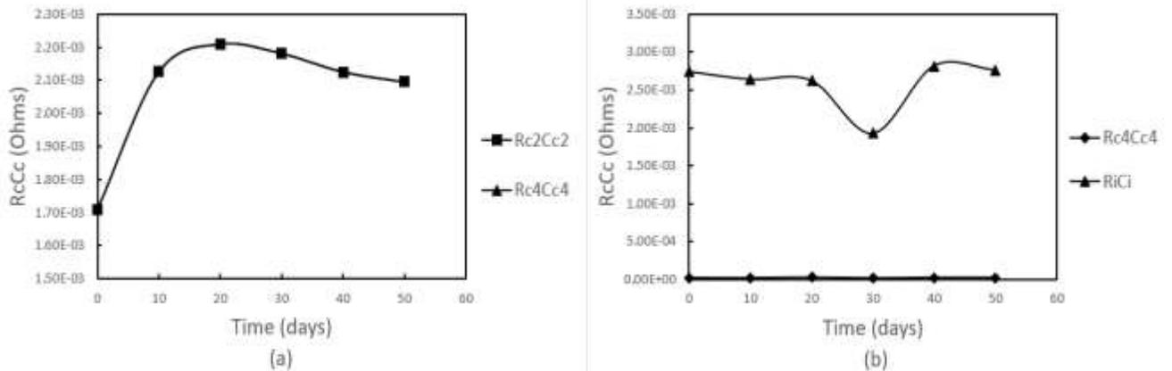
**Figure 13 Variation of corrosion index of (a) C2-C4 probe configuration and (b) M1-C4 probe configuration over time**
