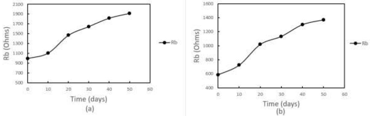
**Figure 10 Variation of bulk resistance of (a) C2-C4 probe configuration and (b) M1-C4 probe configuration over time**
