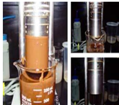
Figure 3: Cleaning efficiency test of Bentonite Drilling muds using Viscometer.
