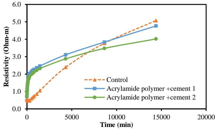
**Figure 1: Electrical resistivity during curing time**
