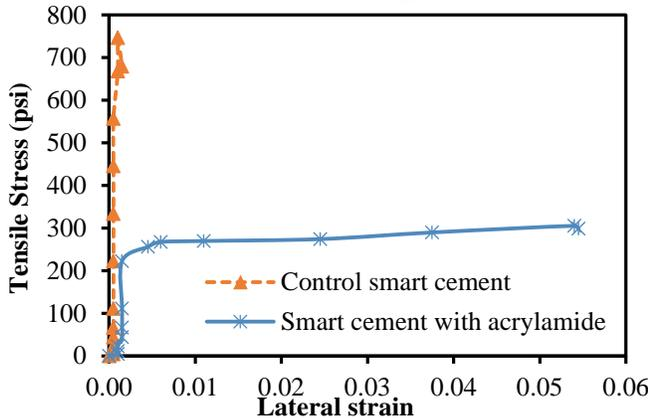
**Figure 2: Splitting tensile test of the smart cement and polymer modified smart cement**
