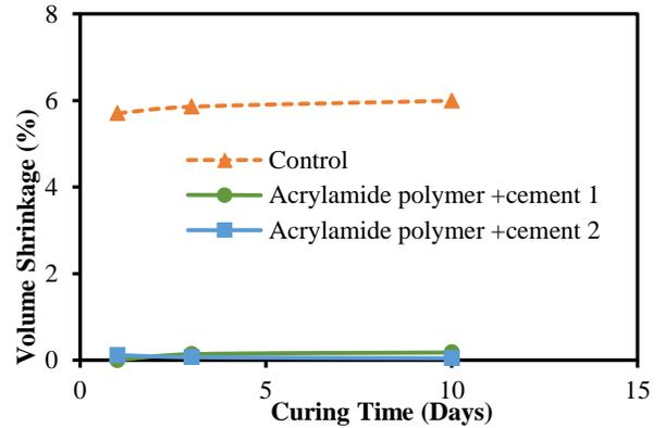
**Figure 5: Volume shrinkage of polymer modified smart cement with curing time**
