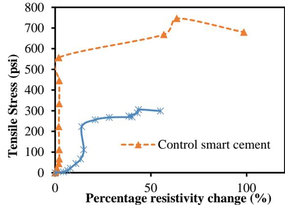
**Figure 3: Piezoresistive behavior of the smart cement and polymer modified smart cement.**
