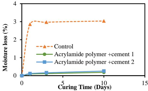
**Figure 4: Moisture loss of polymer modified smart cement with curing time**
