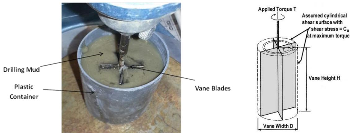
**Figure 1. Laboratory Vane Shear Device with Schematic Idealization.**
