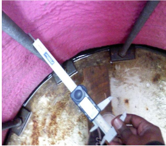
Figure 1: Vernier caliper used for deformation measurement
