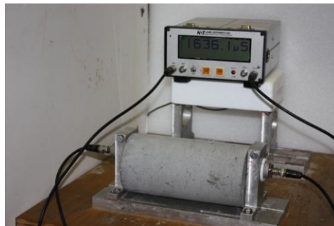
Fig. 1. Ultrasonic pulse velocity meter (V-meter) test with direct transmission test.
