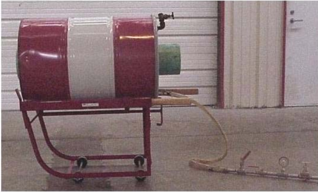
Figure 1. ♦ Model Test on Leaking Pipe Joint
