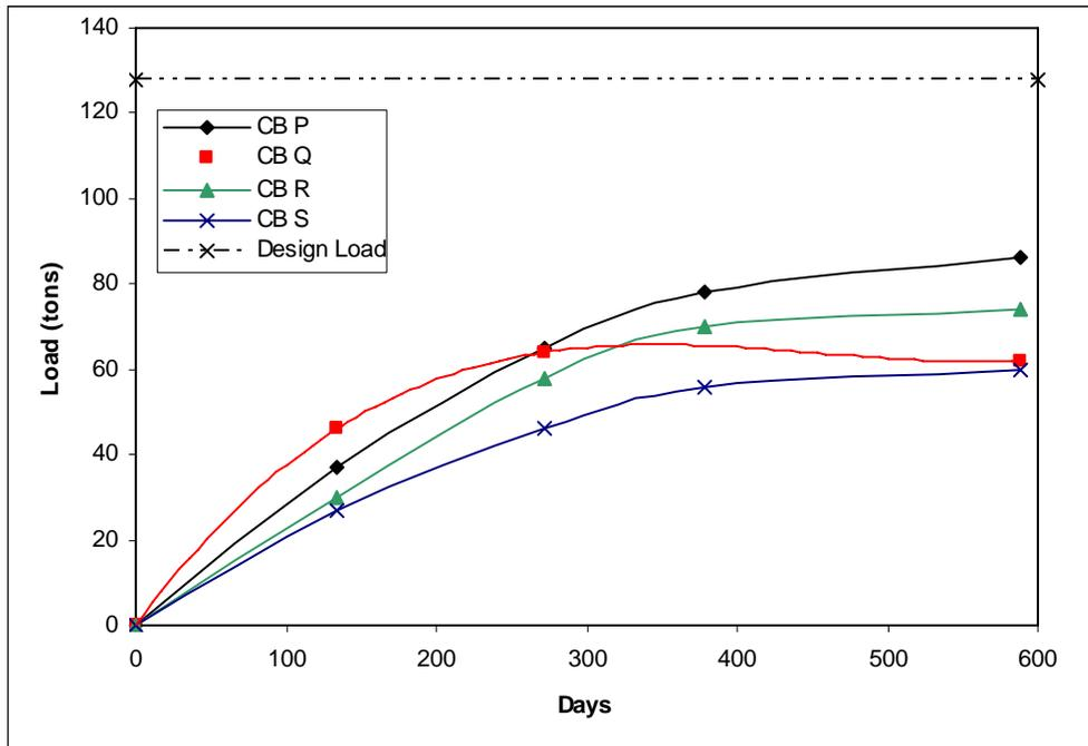
**Fig. 8 Load carried by the CB service piles**
