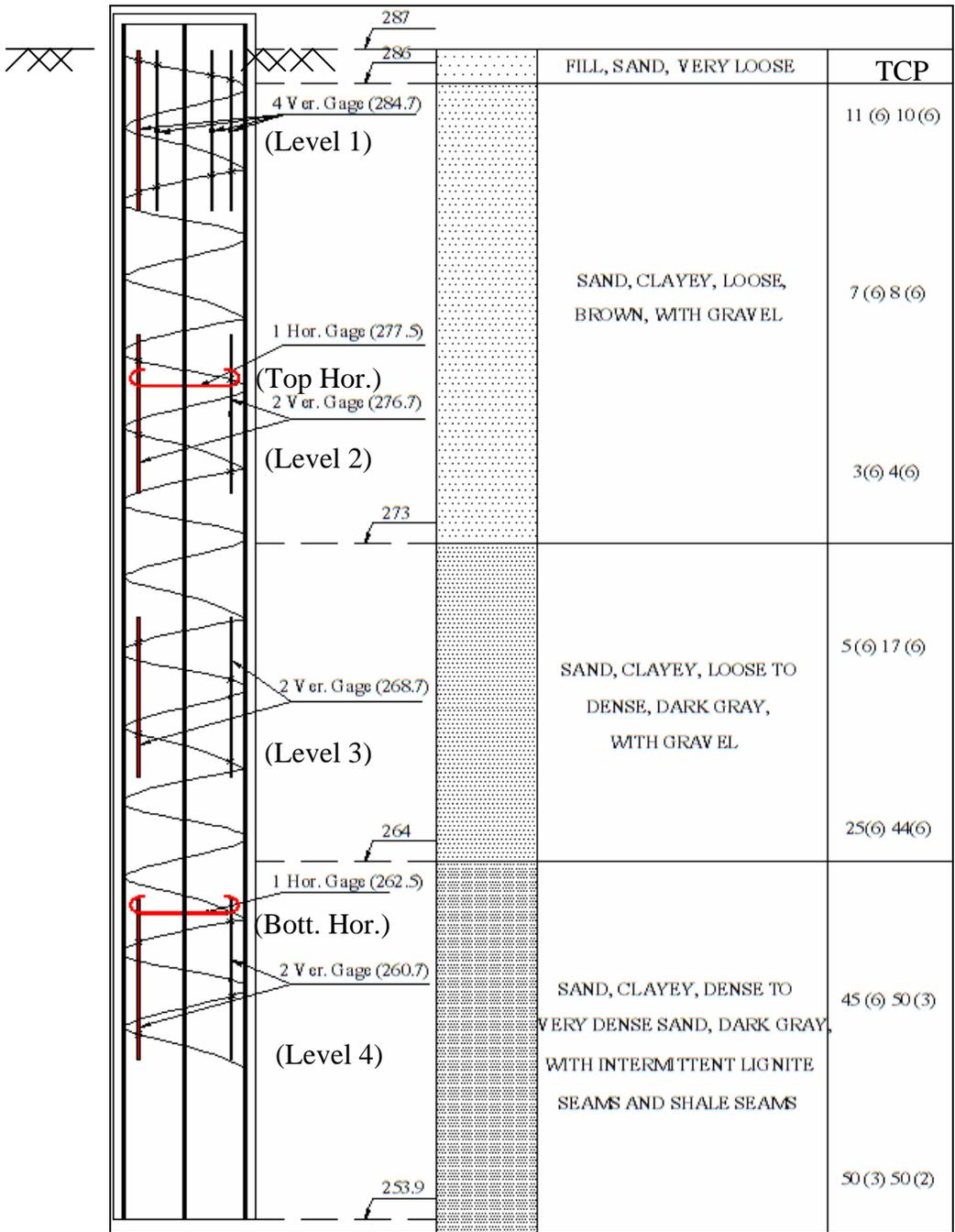
**Fig. 1 Instrumentation and Geotechnical Profile at ECB Site**
