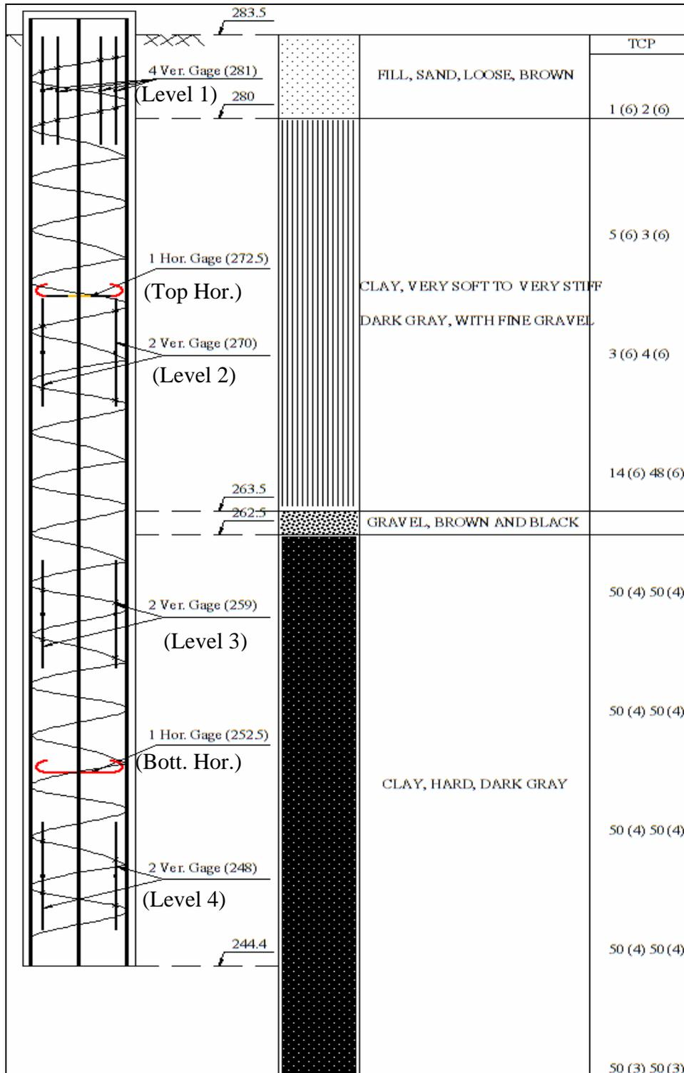
**Fig. 2 Instrumentation and Geotechnical Profile at ECB Site**
