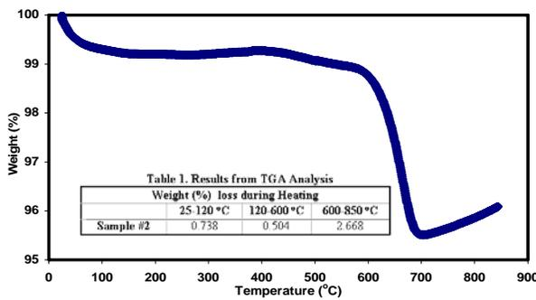
**Figure 4. TGA analysis on clay soil (sample #2)**
