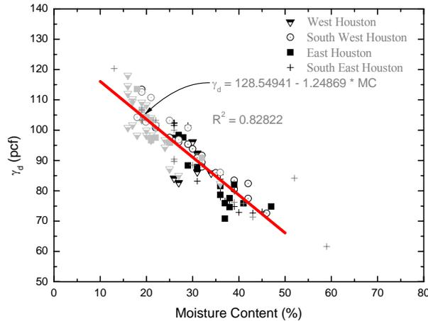
Figure 9. Variation of dry density with moisture Content
