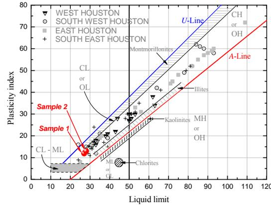
**Figure 8. Plasticity chart with the soil data**
