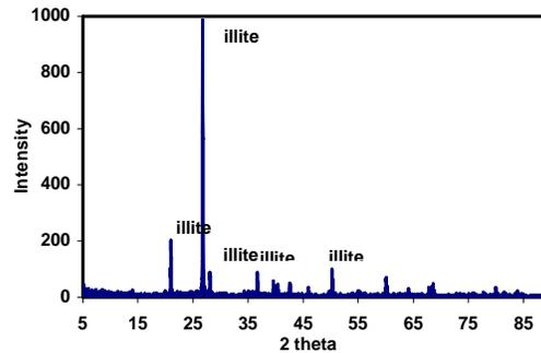
**Figure 5. XRD analysis of clay soil (sample #2)**
