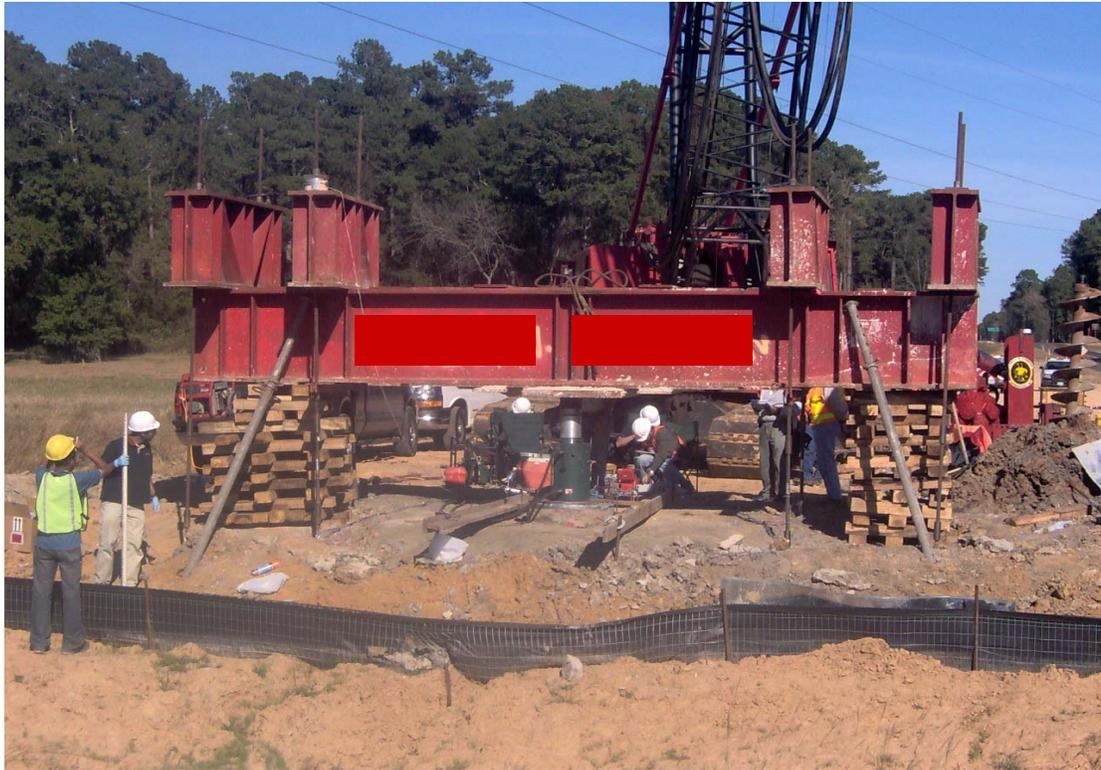
**Figure 9. Load Test on 760 mm diameter ACIP Pile using a single beam with 8 reaction piles for a designed capacity of over 5 MN**
