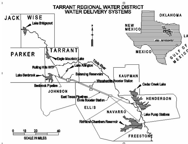
twenty percent of the total supply, and release water down the Trinity River to Tarrant County. Water from Cedar Creek is pumped using a 72-inch diameter, sixty-eight mile long pipeline and an 84-inch diameter six-mile long pipeline to Tarrant County. Water is pumped from Richland Chambers in a 90-inch diameter seventy-two mile long pipeline and a 108-inch diameter six-mile long pipeline to Tarrant County. Since Cedar Creek and Richland
