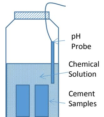
**Figure 1: Schematic diagram of the chemical resistance test**
