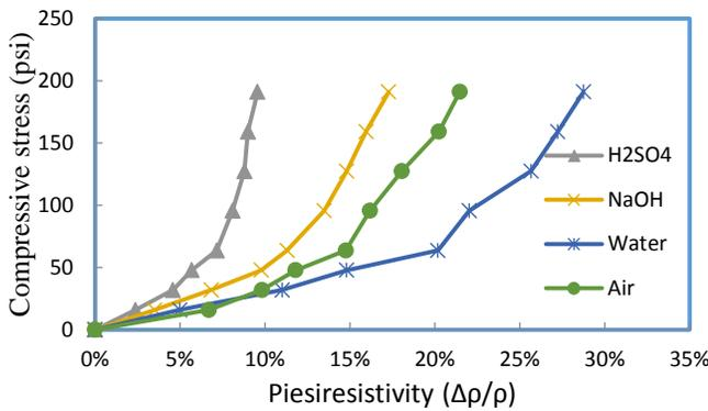
Figure 3: Compressive behavior of ultra fine cement
