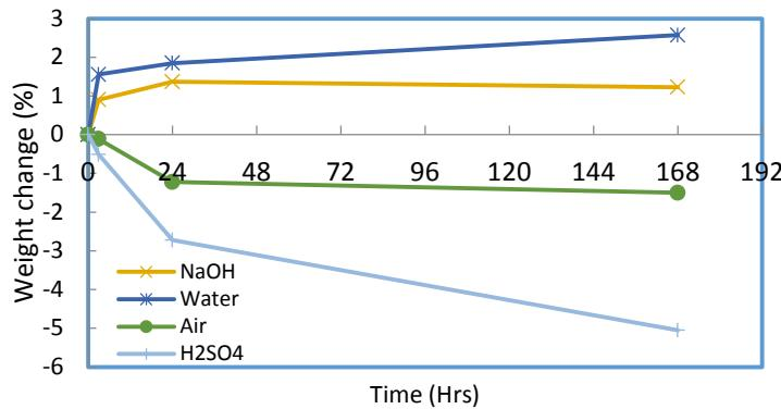
Figure 2: Weight change with time for fine cement
