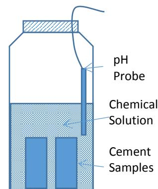
Figure 1: Schematic diagram of the chemical resistance test
