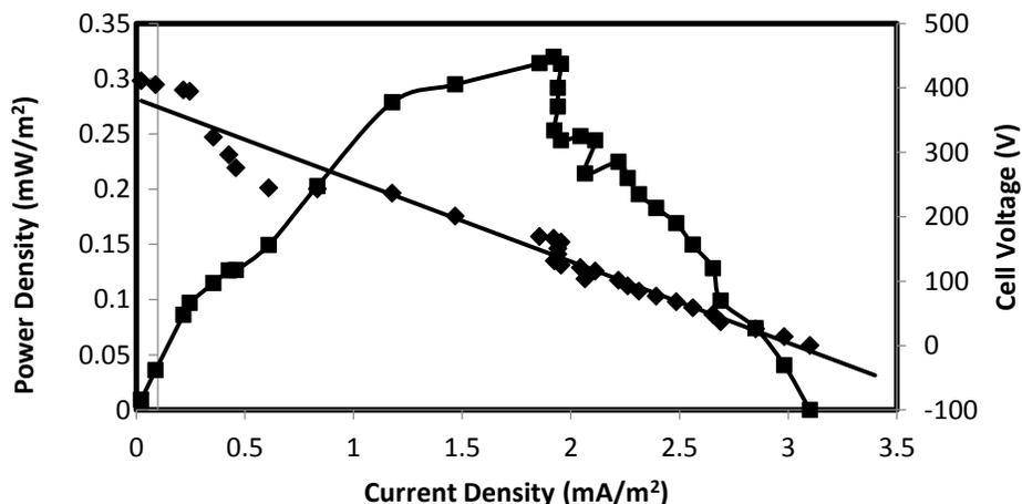
Fig.2 Power Density and Polarization Plot of Microbial Fuel Cell with Ni nanoparticles on Cathode Surface
