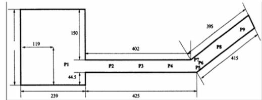
Fig. 3: Dam break problem in a 45° channel bend.
