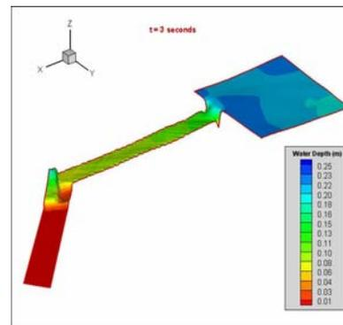
Fig. 5: 3D view of wave propagation in the channel at t =3secs.
