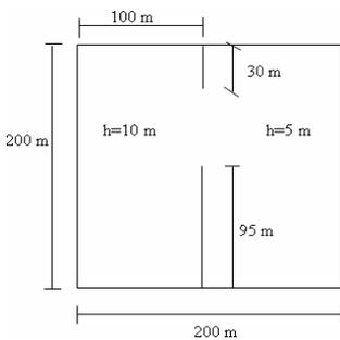
Fig. 1: Dam break problem in a 200m x 200 m domain.
