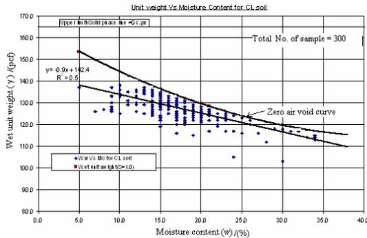
Fig.1 Variation of unit weight with moisture content for CL soil
